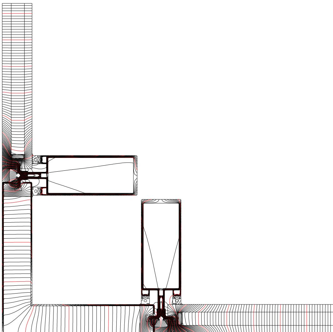
**Dew point isotherm diagram****Line at dew point equivalent to 40 % RH shown i.e. 6.01 deg C**
