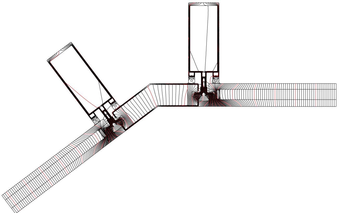
**Dew point isotherm diagram****Line at dew point equivalent to 40 % RH shown i.e. 6.01 deg C**
