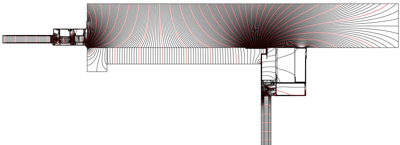
**Dew point isotherm diagram****Line at dew point equivalent to 40 % RH shown i.e. 6.01 deg C**
