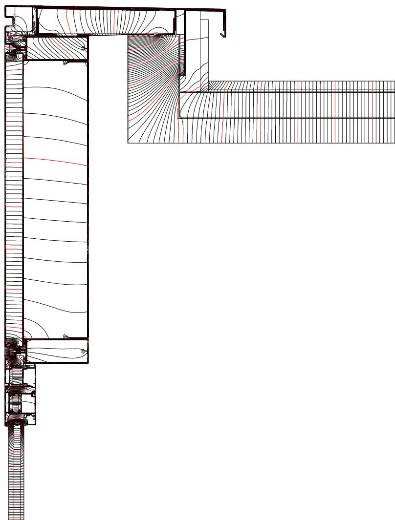
**Dew point isotherm diagram****Line at dew point equivalent to 40 % RH shown i.e. 6.01 deg C**
