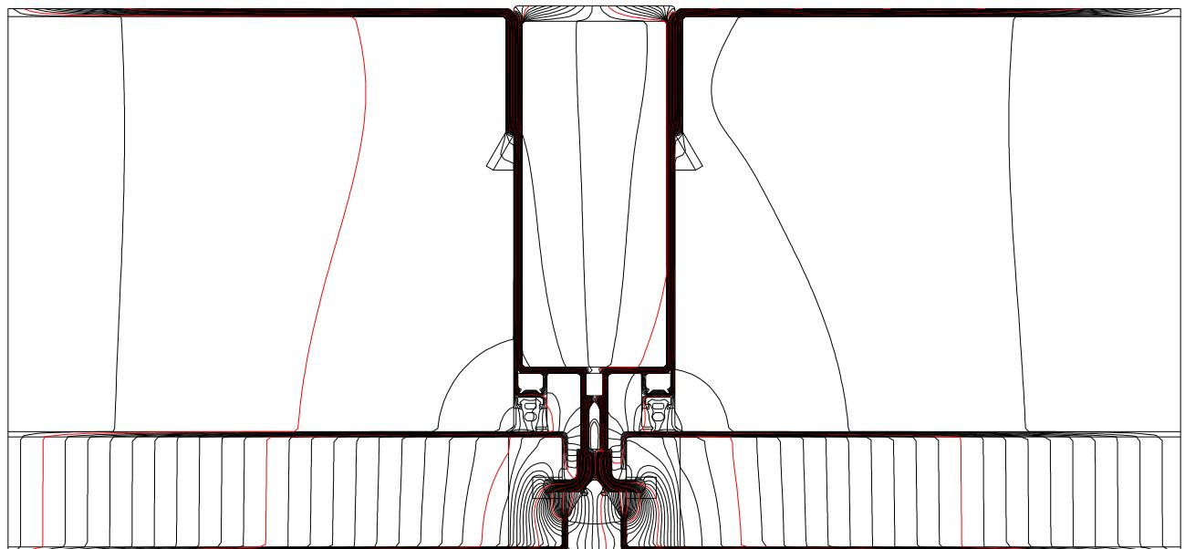
**Dew point isotherm diagram****Line at dew point equivalent to 40 % RH shown i.e. 6.01 deg C**
