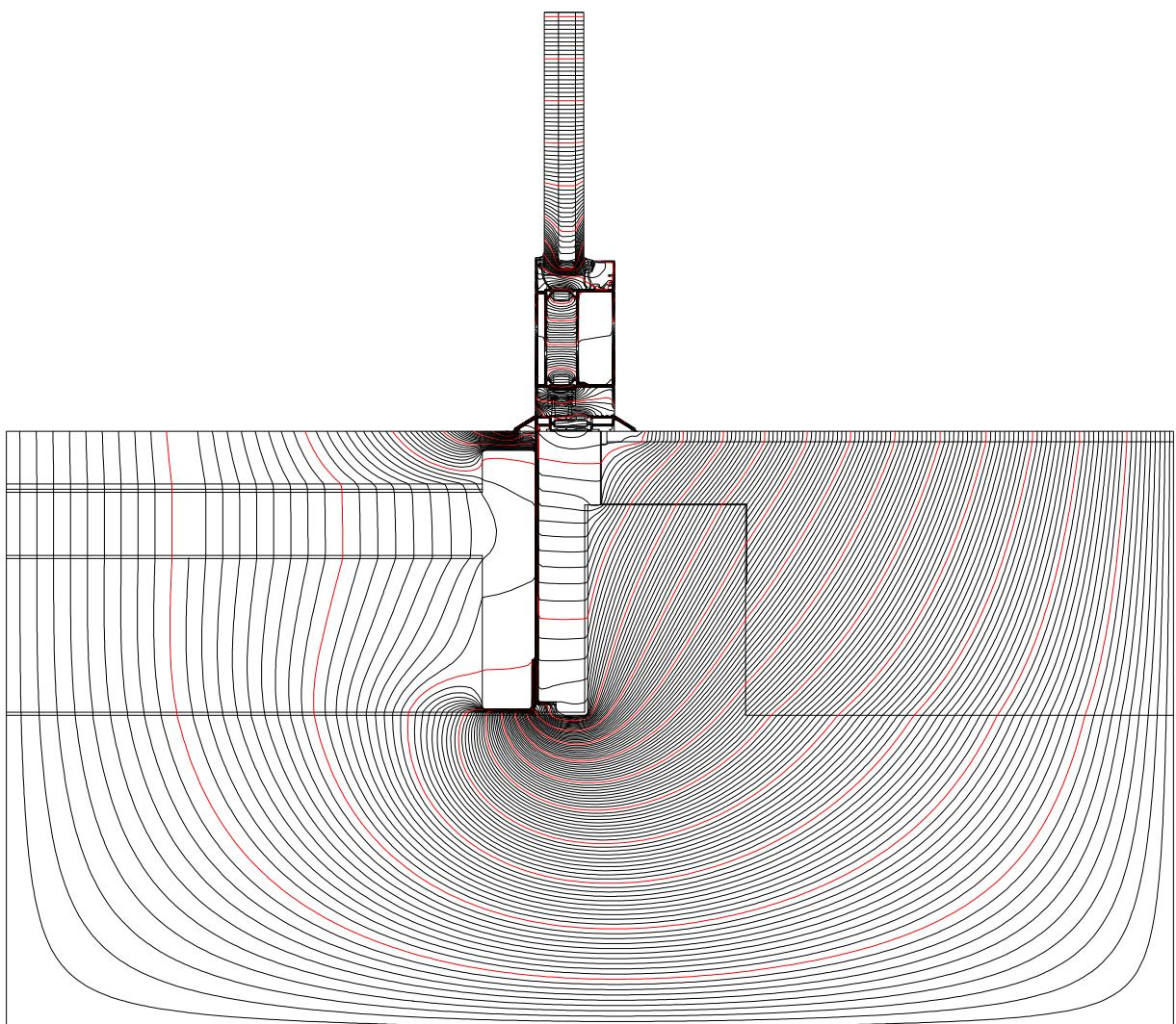
**Dew point isotherm diagram****Line at dew point equivalent to 40 % RH shown i.e. 6.01 deg C**
