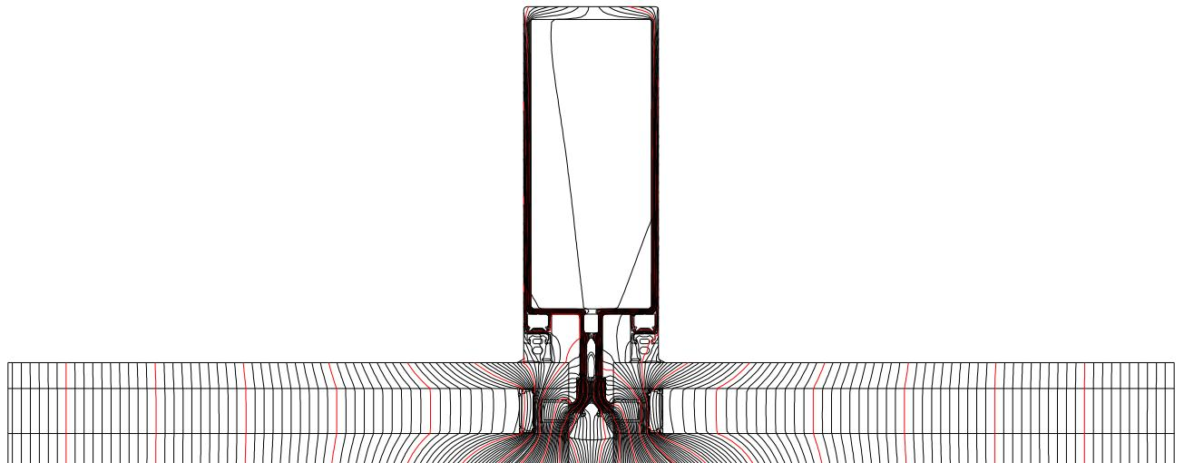
**Dew point isotherm diagram****Line at dew point equivalent to 40 % RH shown i.e. 6.01 deg C**
