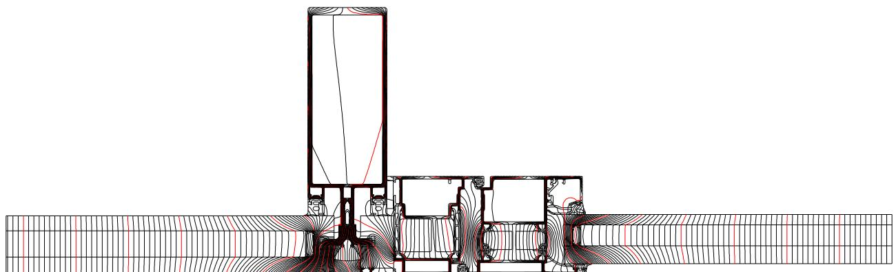
**Dew point isotherm diagram****Line at dew point equivalent to 40 % RH shown i.e. 6.01 deg C**
