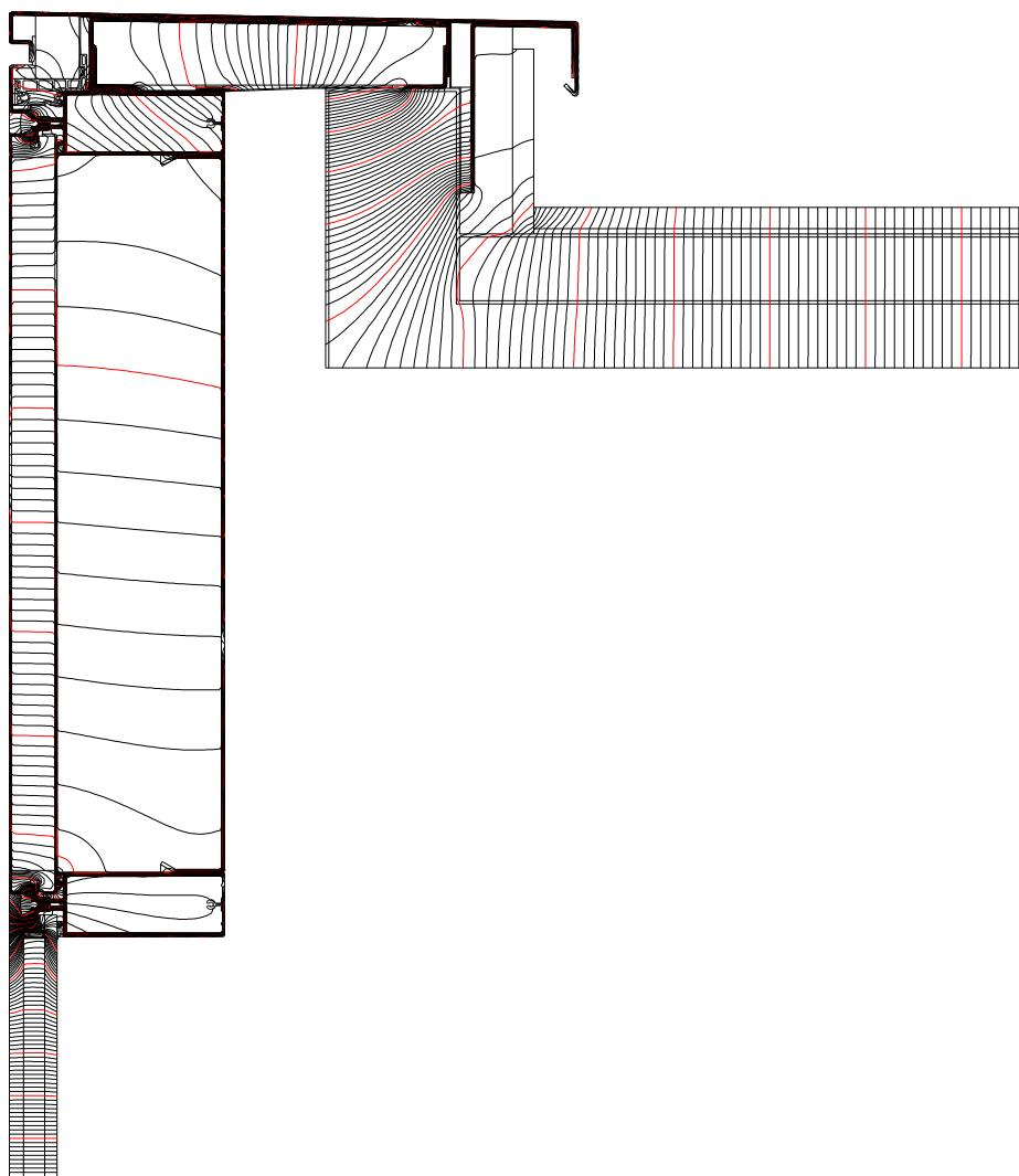
**Dew point isotherm diagram****Line at dew point equivalent to 40 % RH shown i.e. 6.01 deg C**
