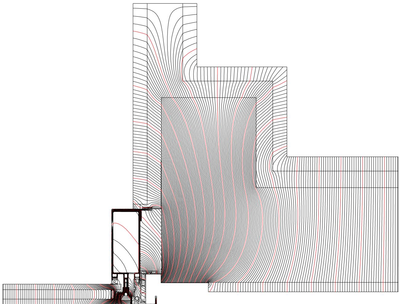
**Dew point isotherm diagram****Line at dew point equivalent to 40 % RH shown i.e. 6.01 deg C**
