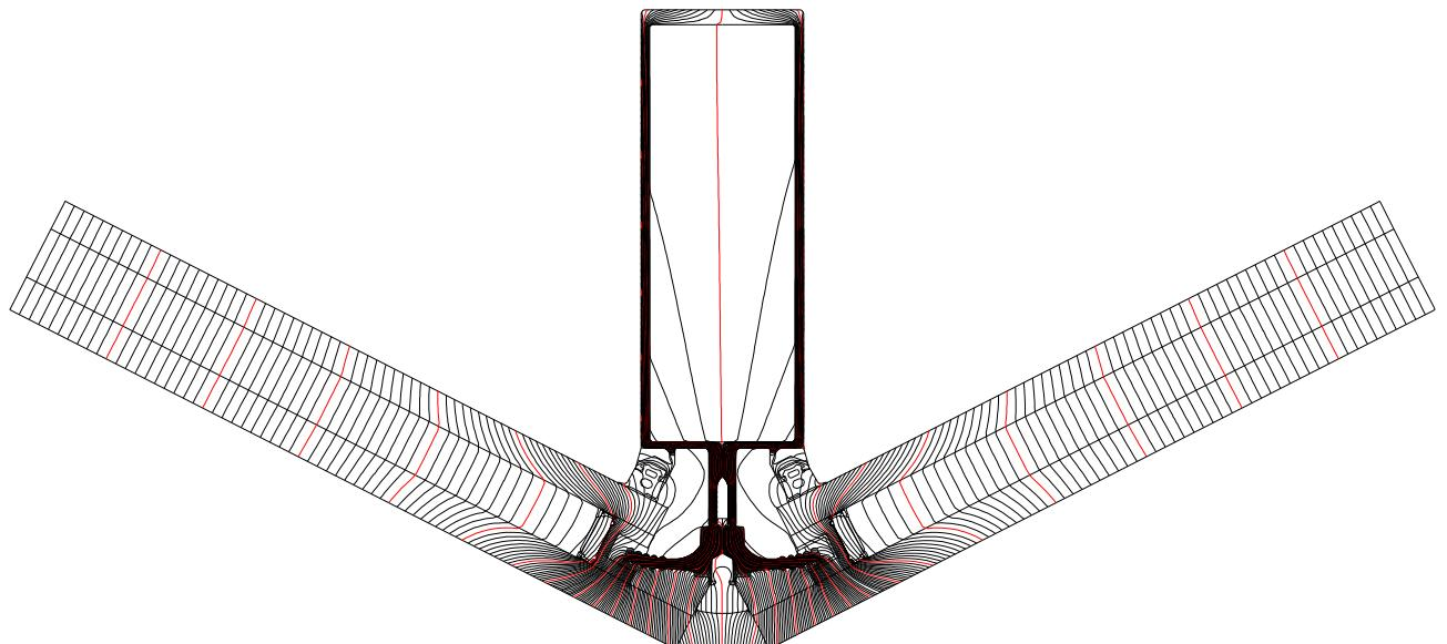
**Dew point isotherm diagram****Line at dew point equivalent to 40 % RH shown i.e. 6.01 deg C**
