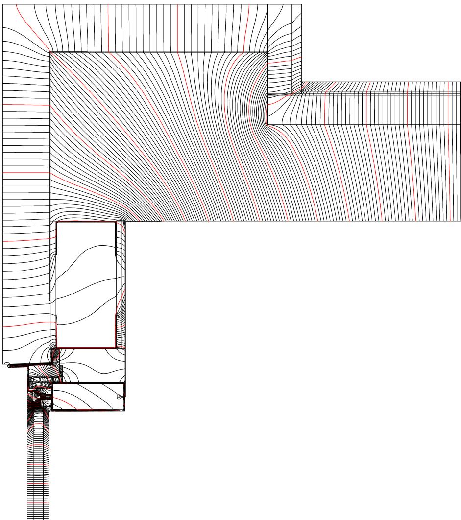
**Dew point isotherm diagram****Line at dew point equivalent to 40 % RH shown i.e. 6.01 deg C**
