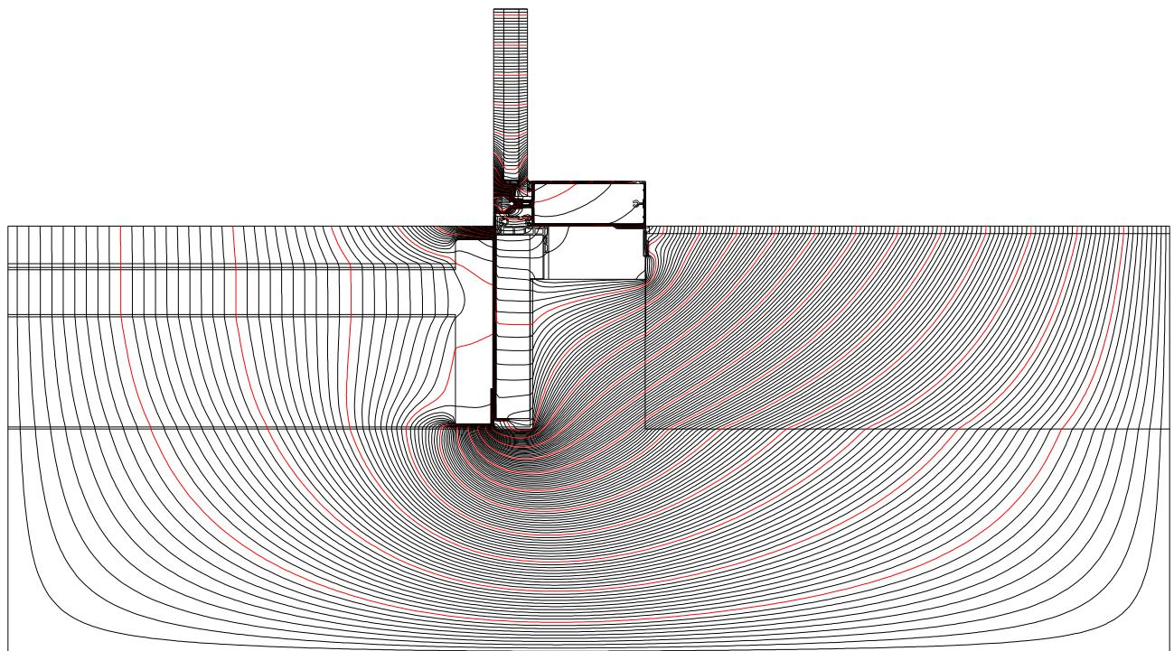
**Dew point isotherm diagram****Line at dew point equivalent to 40 % RH shown i.e. 6.01 deg C**
