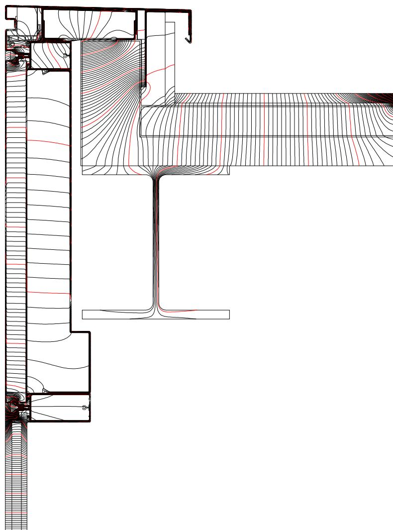
**Dew point isotherm diagram****Line at dew point equivalent to 40 % RH shown i.e. 6.01 deg C**
