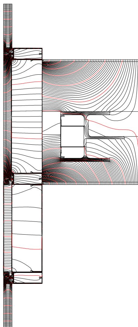
**Dew point isotherm diagram****Line at dew point equivalent to 40 % RH shown i.e. 6.01 deg C**
